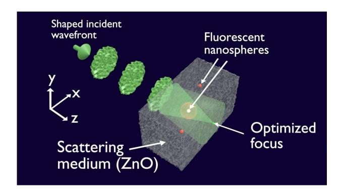
Figure 1. An opaque material that is illuminated with a laser beam (green) whose wavefronts are spatially shaped. Part of the shaped incident light is focused at the back surface of the opaque medium, and part of the light is randomly scattered in a surrounding diffuse background. Isolated fluorescent nanospheres (red dots) serve to "report" the energy density of the green light via the red intensity that is collected in the Twente experiment. Credit: University of Twente
