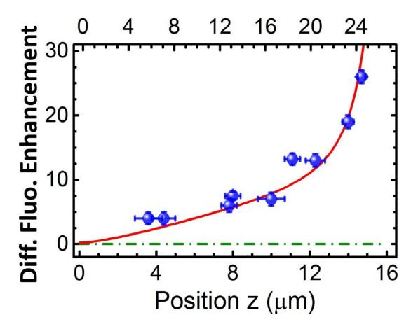
Figure 2. Differential fluorescence enhancement probed by nanospheres at different depths z, while shaping the incident wavefront of light to reach a focused target at the sample back surface (compare Fig. 1). The enhancement increases with depth z, meaning that the photons have a much greater density much deeper inside the 3D white paint. Credit: University of Twente
