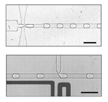
Cells made from water in oil: Using microfluidics technology, a Franco-German research team first generates tiny droplets (top) into which the components of a simple metabolism are then injected (bottom). The bar corresponds to 100 micrometers. Credit: Nature Communications 2018
