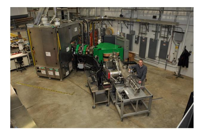
A team of ORNL researchers including Brian Egle (pictured) developed an electromagnetic isotope separator system that was used to produce ruthenium-96. Credit: Oak Ridge National Laboratory
