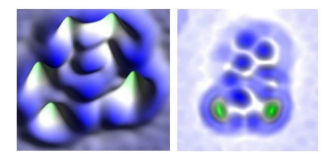
On left: AFM image using a CO-functionalized tip of 5,6,8-trimethyl-2,3-dihydro-1H-cyclopenta(b)naphthalene, a molecule found in the deep ocean. On right: AFM image using a CO-functionalized tip of a molecule found in the deep North Pacific Ocean.
