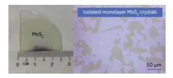
Two-dimensional monolayer  $MoS_2$  was grown on sapphire (left). The optical microscope image on the right shows isolated monolayer  $MoS_2$  crystals at the periphery of the film. Adapted with permission from Ref 1. Copyright (2018) American Chemical Society.
