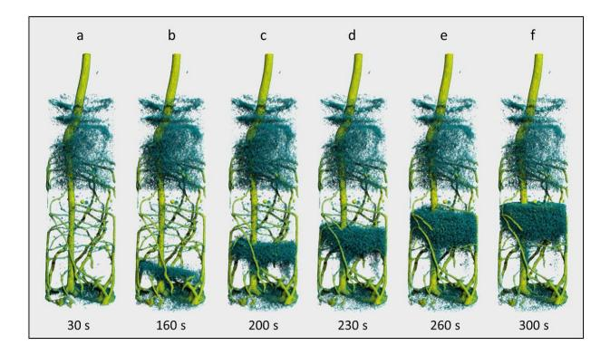
Sequential tomography of a lupin root (yellowish green) after deuterated water (D2O) was introduced from below. The rising water front (H2O, dark blue) is displaced by the D2O from below over the course of time. Credit: Christian Tötzke/ University of Potsdam
