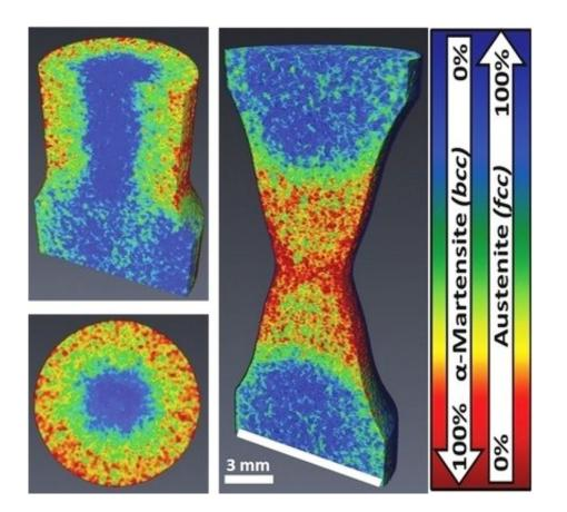
Neutron tomography shows how torsion (images left) and tensile forces (image right) are changing the distribution of different crystalline phases. Credit: HZB/Wiley VCH
