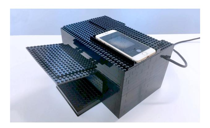
Made from Lego bricks and a smart phone, a device is connected to free software and utilizes the phone's camera to identify and detect nerve agents, like VX and sarin. Credit: University of Texas at Austin
