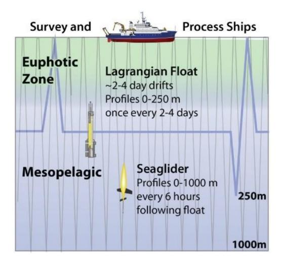
The UW researchers will use drifting, or Lagrangian, floats that adjust their buoyancy to move up and down through the sunlit euphotic zone. The UW team will use ocean drones called Seagliders to survey deeper water. Credit: Eric D'Asaro and Craig Lee/University of Washington
