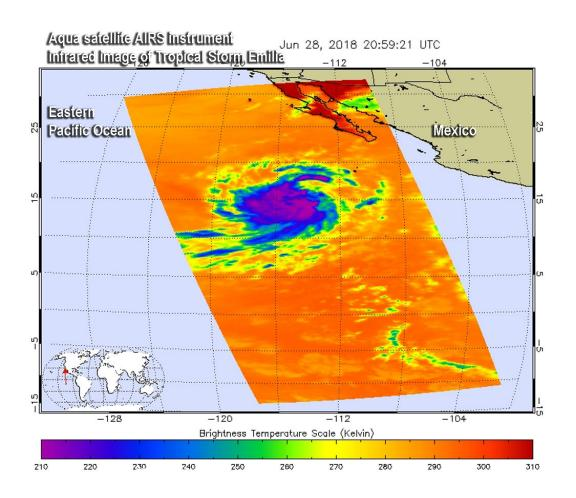
On June 28 at 4:59 p.m. EDT (2059 UTC) the AIRS instrument aboard NASA's Aqua satellite showed powerful storms with very cold cloud top temperatures (purple) in excess of minus 63 degrees Fahrenheit. Credit: NASA JPL, Heidar Thrastarson
