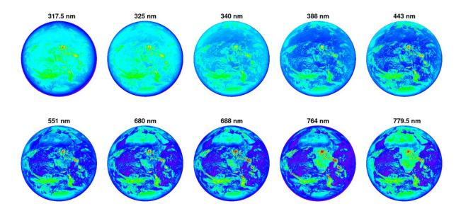
This image shows the sunlit side of Earth, observed in 10 wavelengths by the EPIC instrument aboard the DSCOVR satellite. Each image shows the same snapshot of Earth in a different wavelength. The specific wavelength bands are indicated above each image. Credit: NASA/NOAA
