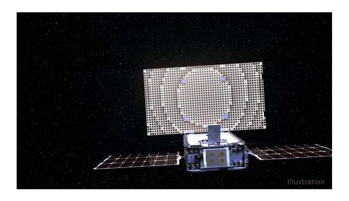
An artist's concept of one of NASA's MarCO CubeSats. The twin MarCOs are the first CubeSats to complete a trajectory correction maneuver, firing their thrusters to guide themselves toward Mars. Credit: NASA/JPL-Caltech
