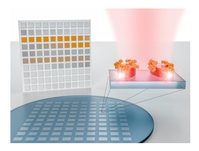
The authors show a pixelated sensor metasurface for molecular spectroscopy. It consists of metapixels designed to concentrate light into nanometer-sized volumes in order to amplify and detect the absorption fingerprint of analyte molecules at specific resonance wavelengths. Simultaneous imaging-based readout of all metapixels provides a spatial map of the molecular absorption fingerprint sampled at the individual resonance wavelengths. This pixelated
