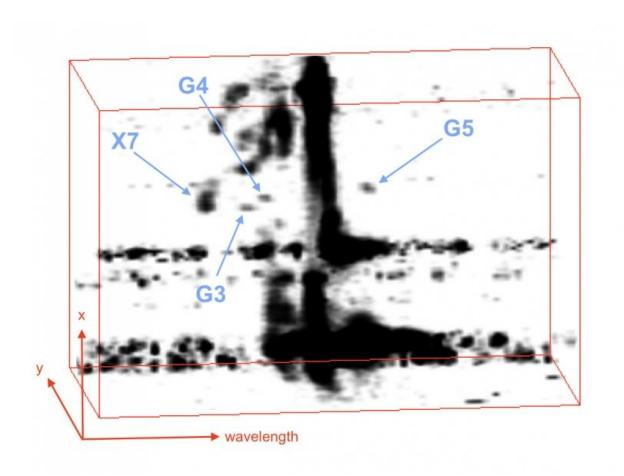
This 3-D spectro-imaging data cube was produced using software called OsrsVol, short for OSIRIS-Volume Display. W. M. Keck Observatory Science Operations Lead Randy Campbell developed this custom volume rendering tool to separate G3, G4, and G5 from the background emission. Once the 3-D analysis was performed, the team could clearly distinguish the G-objects, which allowed them to follow their movement and see how they behave around the
