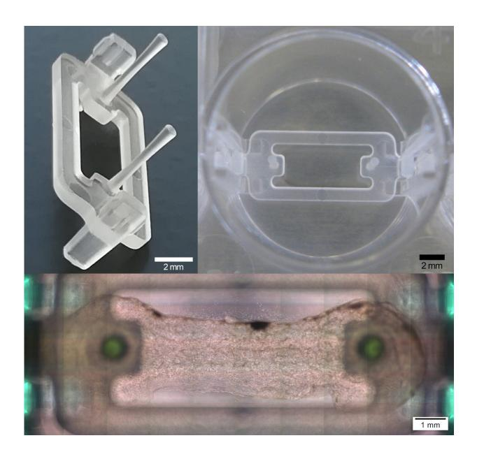
Postholder insert for the printing of dumbbell-shaped muscle-tendon tissues in a
