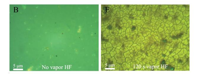
A microscopic look at graphene before (left) and after the VHF exposure is applied for 120 seconds. Credit: KTH
