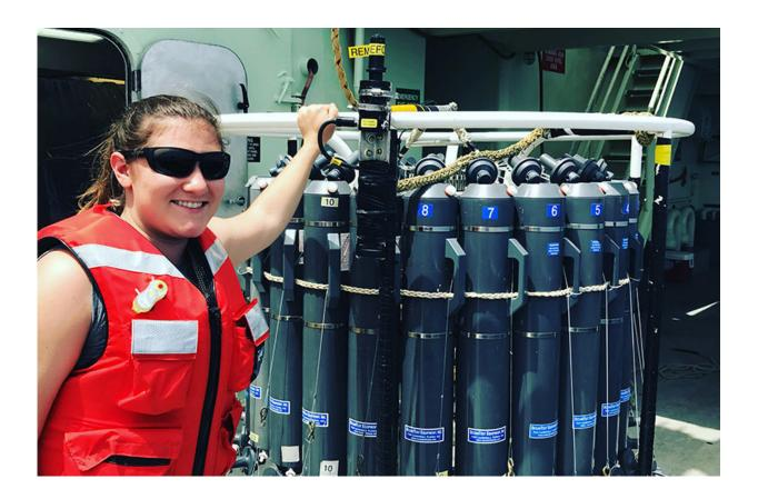
Graham, aboard the RV Atlantis, prepares to deploy a CTD Rosette that is used to determine at which depths to collect ocean water samples. Credit: Babak Hassanzadeh
