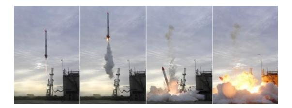
This combination of photos shows the launch of a Japan's privately developed rocket, MOMO-2, from left to right, fails in Taiki, northern island of Hokkaido, Japan, Saturday, June 30, 2018. According to Kyodo News, the launch failed Saturday, as the rocket crashed to the ground and burst into flames seconds after liftoff, its developer said. (Masanori Takei/Kyodo News via AP)
