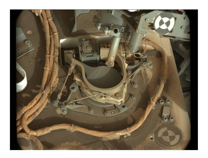
The drill bit of NASA's Curiosity Mars rover over one of the sample inlets on the rover's deck. The inlets lead to Curiosity's onboard laboratories. This image was taken on Sol 2068 by the rover's Mast Camera (Mastcam). It has been white balanced and contrast-enhanced. Credits: NASA/JPL-Caltech/MSSS
