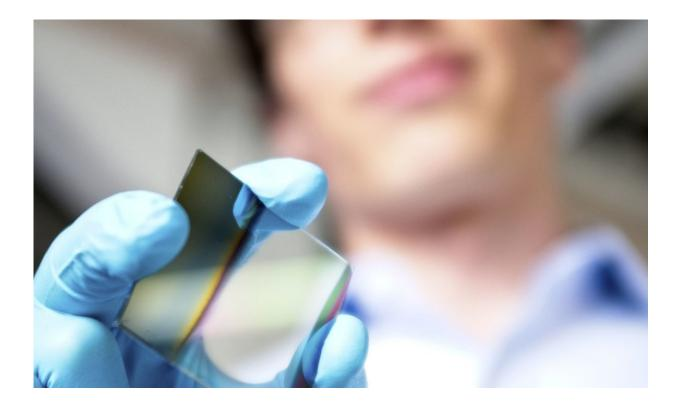
Sebastian Siol showing a sample of heterostructural oxides, which could be a promising coating for smart windows. Credit: EMPA
