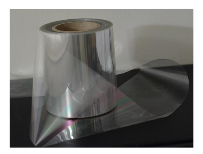
This photo shows nanocellulose-coated PET film. Purdue University researchers created a new manufacturing process using cellulose nanocrystals as advanced barrier coatings for food packaging. Credit: Purdue University
