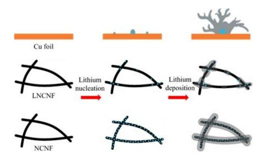
Schematic diagram of lithium nucleation and deposition behavior on Cu foil, low nitrogen-doping level carbon nanofiber framework and high nitrogen-doping level carbon nanofiber framework. Credit: ©Science China Press
