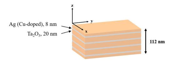
Cross-sectional view of the hyperbolic metamaterial examined in the new study shows layers of copper-doped silver and tantalum pentoxide. Credit: NIST
