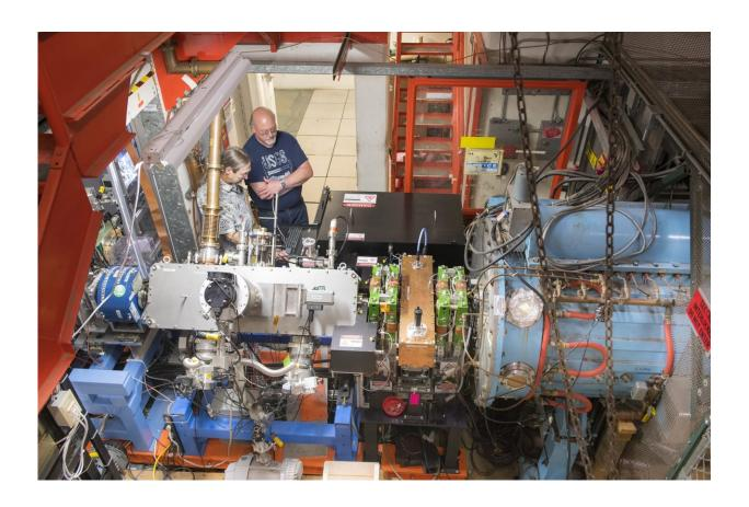
David Johnson, left, and Todd Johnson work on the recently installed laser notcher in the Fermilab accelerator complex. The laser notcher, the first application of its kind in an in-production particle accelerator, has helped boost particle beam production at the lab. Credit: Reidar Hahn
