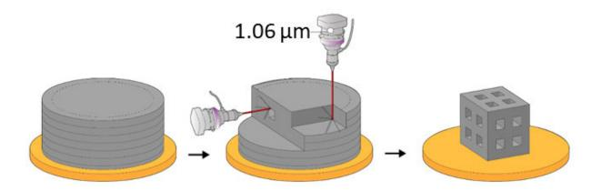
Rice University scientists have layered laser-induced graphene and built a prototype that shapes the resulting 3-D blocks into sophisticated shapes. The foam offers new possibilities for energy storage and flexible electronic sensor applications. Credit: Tour Group/Rice University
