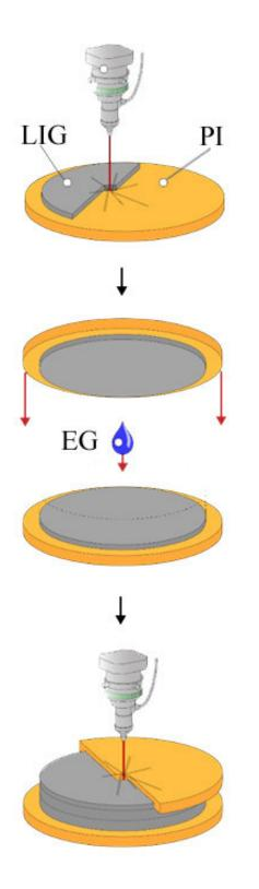
Rice University scientists are making 3-D laser-induced graphene (LIG) foam through an automated process that begins by turning the top layer of a polyimide (PI) sheet into graphene (top), stacking another layer on top (center) with
