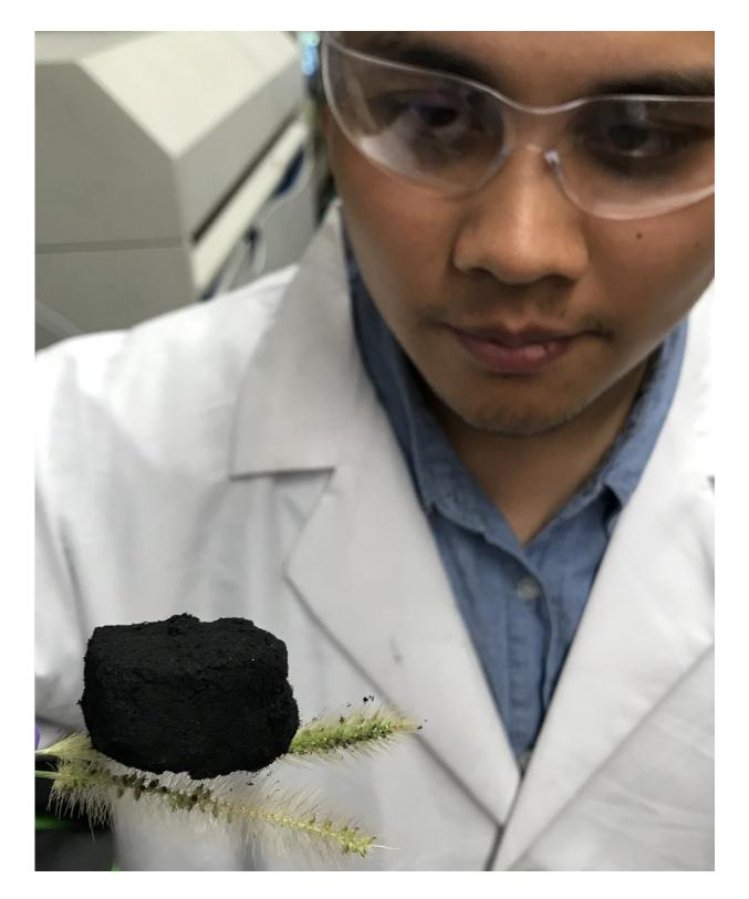
Rice University graduate student Duy Xuan Luong suspends a three-dimensional block of laser-induced graphene atop two willows. The lab uses an industrial
