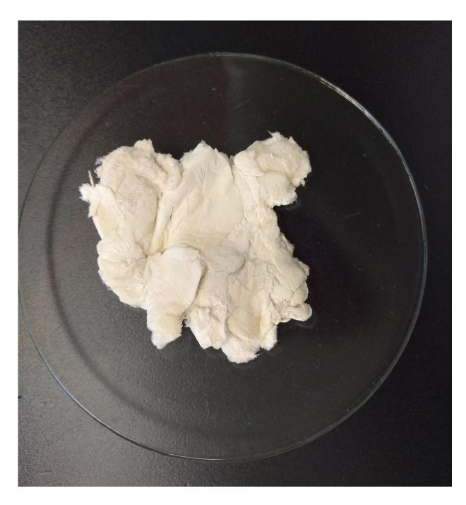
Chitosan, purified from insect skins. Credit: Fraunhofer Institute for Interfacial Engineering and Biotechnology IGB
