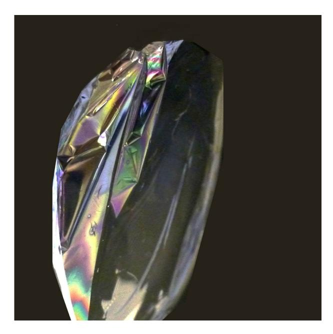
Chitosan is able to form films, which is important for its use as sizing agent. Credit: Fraunhofer Institute for Interfacial Engineering and Biotechnology IGB
