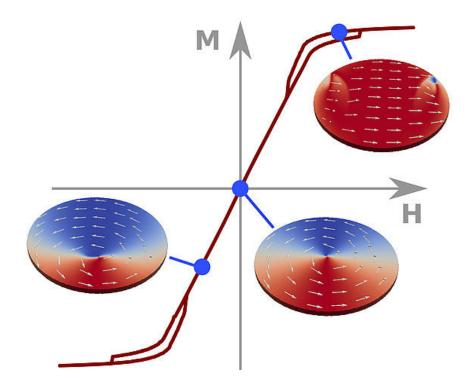
The position of the center of the vortex is proportional to the applied magnetic field and serves as a reproducible and precise measurement variable. Credit: Dieter Suess et al.
