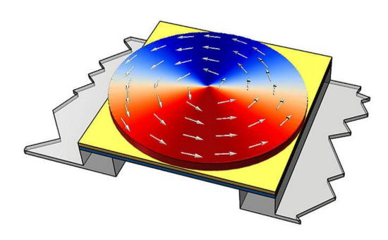
A magnetic sensor in which the magnetic transducer element has a vortex state. Credit: Dieter Suess et al
