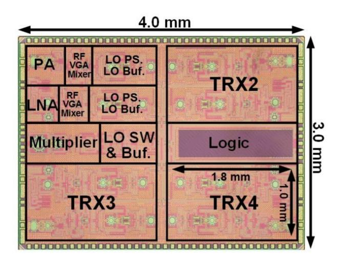
The fabricated transceiver only measures  $3 \text{ mm} \times 4 \text{ mm}$  and consists of four transmitting and receiving elements. The subcomponents of TRX1 are displayed. Credit: IEEE Radio Frequency Integrated Circuits Symposium 2018
