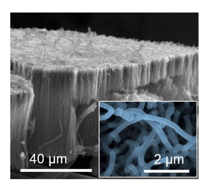
A scanning electron microscopy image of vertically aligned carbon nanotube electrodes coated with titanium disulfide deposited one atomic layer at a time. The magnified inset shows individual titanium disulfide coated carbon nanotube
