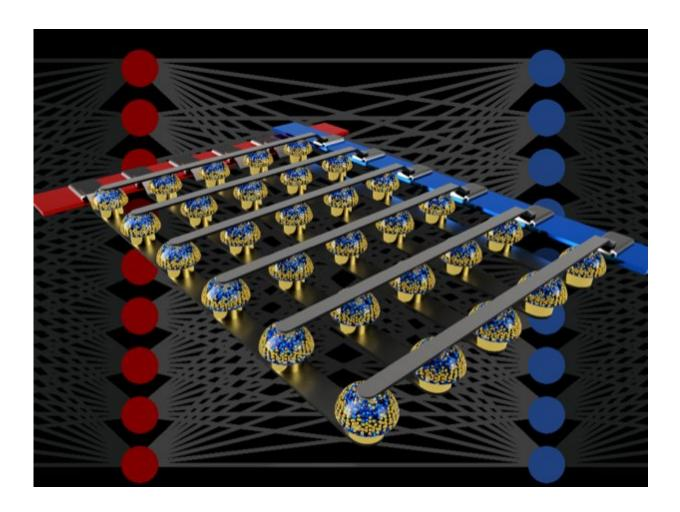
Crossbar arrays of non-volatile memories can accelerate the training of fully connected neural networks by performing computation at the location of the data. Credit: IBM
