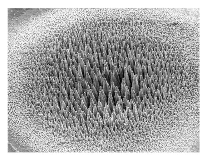
The needle-shaped surface structure of black silicon where needles are made of single-crystal silicon. The nanomaterial is absolutely chemically inert, non-invasive, and could support a strong and non-distorted signal Credit: FEFU
