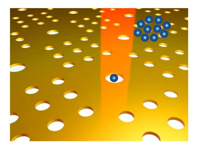
Squeezing light into nano-size volumes is enabled by surface plasmon resonance, a phenomenon that causes molecules to be trapped near the film, making them available for study under powerful microscopes. Credit: Justus Ndukaife/Vanderbilt University
