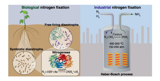
Nitrogen fixation occurs naturally in bacteria containing the nitrogenase enzyme and can be carried out artificially through a high-temperature and high-pressure industrial process that relies on iron-based catalysts and large quantities of hydrogen obtained from natural gas. Source: National Science Foundation workshop report. Credit: Brookhaven National Laboratory
