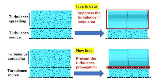
(top) Idea to date: To suppress the turbulence in a high-temperature plasma region it was thought that the turbulence should be suppressed in a large area.(bottom) New idea: It is thought that the turbulence propagation is needed to suppress. Credit: Dr. Katsumi Ida
