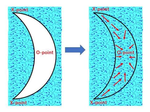
(left) There is no or small turbulence due to the almost zero temperature gradient inside the crescent-shaped magnetic island. (right) Turbulence propagates inside the magnetic island faster than the heat pulse. Credit: Dr. Katsumi Ida
