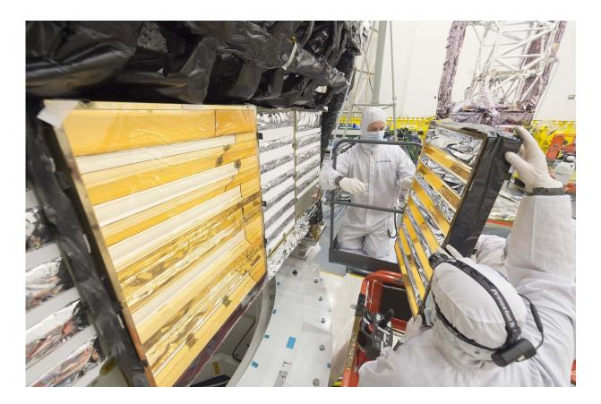
Engineers carefully hold onto a gold-plated baffle as they use a scissor lift to access the back of the integrated science instrument module (ISIM) of NASA's James Webb Space Telescope. They are in the process of reinstalling the baffles, which direct the heat generated by the instrument electronics safely into space and away from any cold areas of the infrared telescope. Credit: NASA/Chris Gunn
