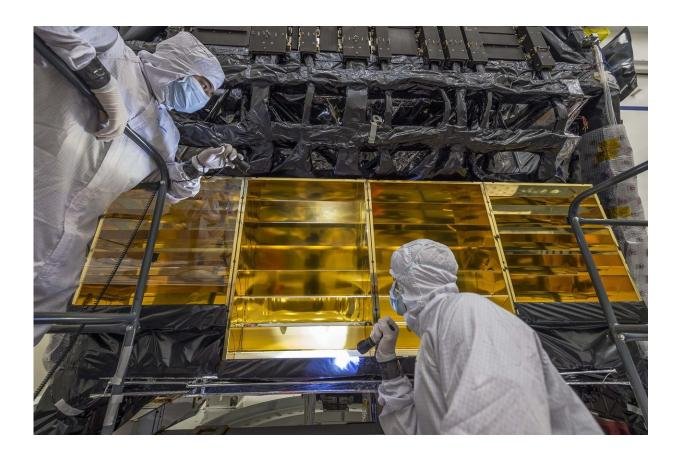
Engineers reinstall one of the gold-plated baffles that helps direct heat away from the integrated science instrument module (ISIM) of NASA's James Webb Space Telescope. The baffles direct the heat generated by the instrument electronics safely into space and away from any cold areas of the infrared telescope. Credit: NASA/Chris Gunn
