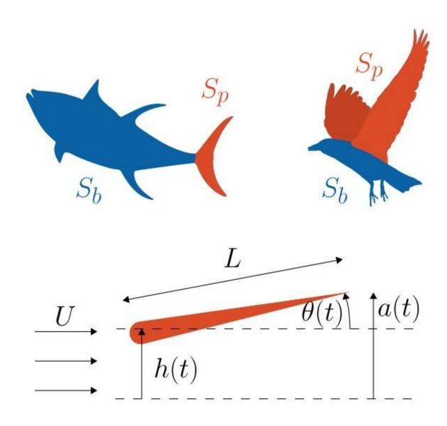
Swimmers and fliers can be decomposed into thrust-producing (orange) and dragproducing (blue) parts, with the propulsor aptly represented by an oscillating
