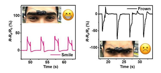
Signals from the electrically conductive hydrogel can clearly distinguish between different facial expressions. Credit: 2018 KAUST
