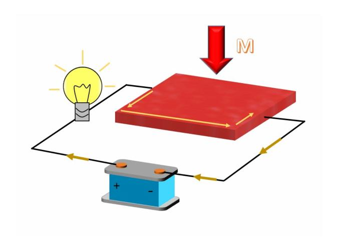
An exotic magnetic insulator conducts electricity along its edges without energy loss. The M stands for magnetization of the magnet, and this GIF shows the magnetization reversal process (red to blue and vice versa). Credit: Wenbo Wang/Rutgers University-New Brunswick
