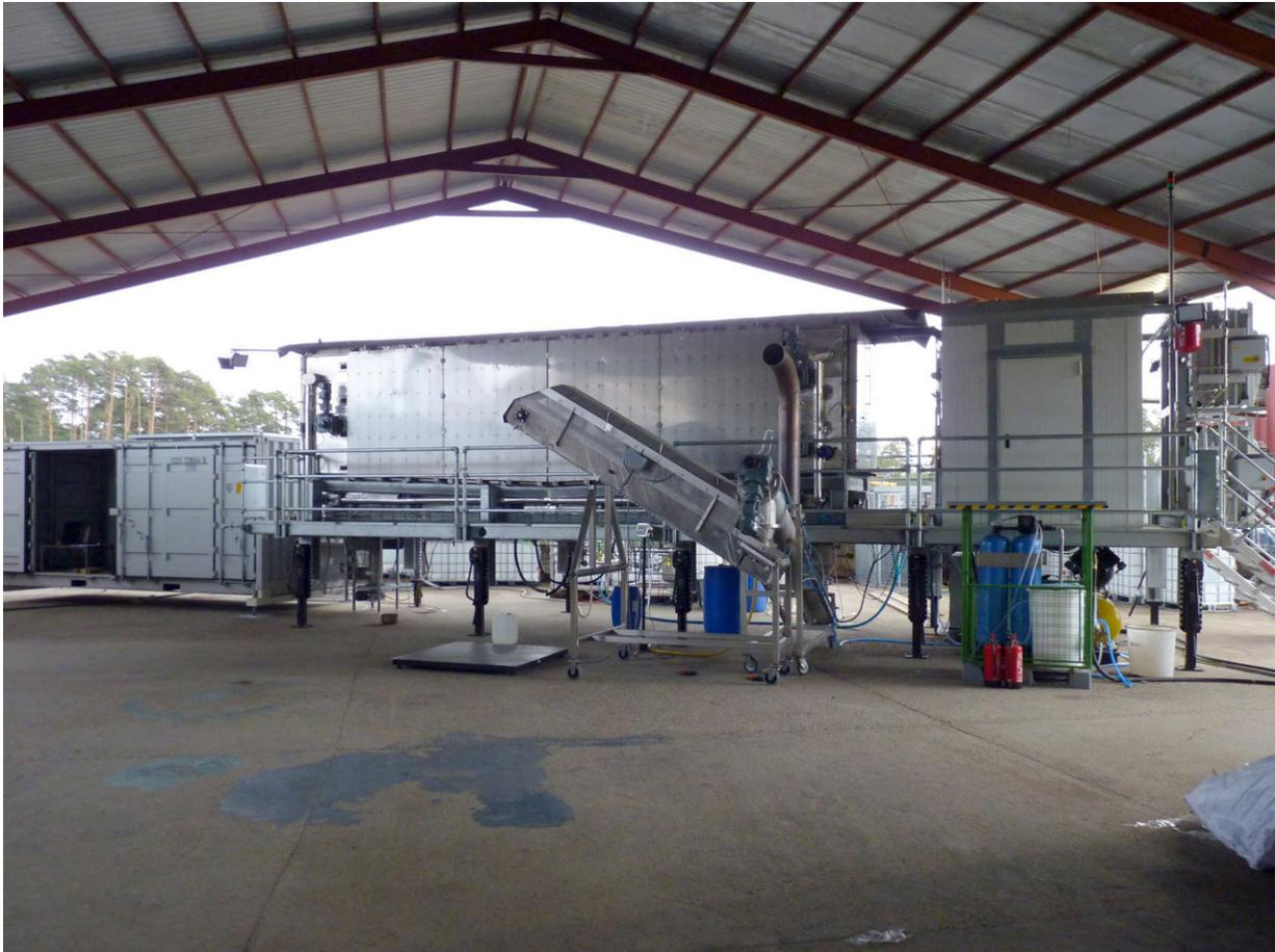
The pilot facility consists of a container with a storage bin and energy center, as well as of a frame that houses the drying and torrefaction reactors, the attachment for extracting solids and the condensers. Credit: Fraunhofer-Gesellschaft
