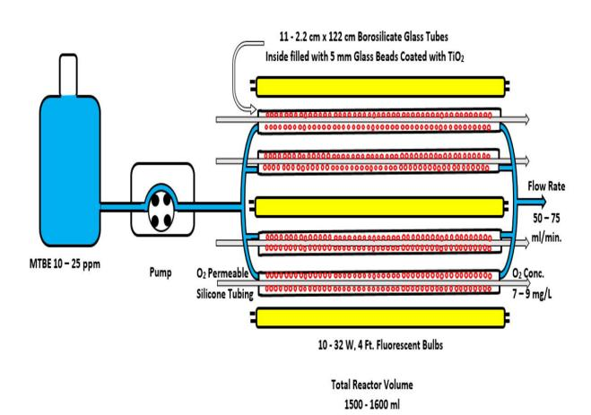
Purdue University researchers developed a series of continuous-flow photoreactors to effectively remove chemical products and compounds from water supplies. Credit: Reynaldo Barreto
