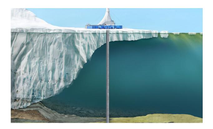
This is a schematic of the drilling rig used to collect the sediment core analyzed by Shakun and colleagues from beneath the Ross Ice Shelf. The drill penetrated 280 feet of ice, 2800 feet of ocean water, and 4200 feet of sediment, recovering a geological history of the Antarctic Ice Sheet stretching back millions of years. Credit: Angie Fox, ANDRILL
