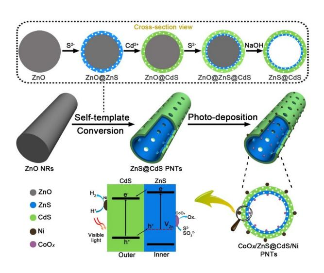
Self-template synthesis of ZnS@CdS PNTs and successive in situ photodeposition synthesis of CoOx/ZnS@CdS/Ni PNTs, and Schematic illustration of photocatalytic H2 production process in CoOx/ZnS@CdS/Ni PNTs. Credit: Science China Press
