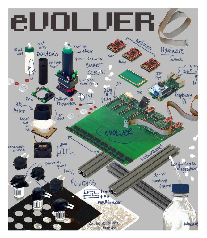
eVOLVER combines the control of automated, continuous cell-culturing systems with the scale of high-throughput systems that grow many cultures at once. Credit: C. Bashor/Rice University
