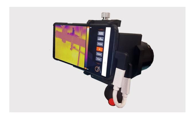
Gas detection camera. Credit: UC3M
