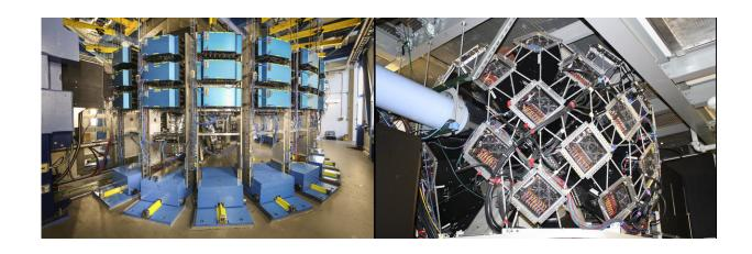
Detectors at SNS and HFIR help researchers study scattered neutrons to better understand the nature of materials. An ORNL team designs detectors tailored to meet the specifications of each instrument, such as the WLS detectors installed at the recently upgraded POWGEN, SNS beamline 11A (left), and the Anger cameras installed at MaNDi, SNS beamline 11B (right). Credit: ORNL/Genevieve Martin
