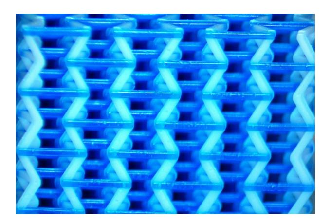
A micro-lattice structure made from different materials. Multi-material programmable additive manufacturing allows for printing materials of different modulus without cross-contamination. Credit: Virginia Tech
