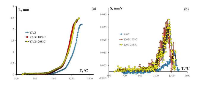
Sintering diagrams for fine-grained YAG-SiC composites: dependencies of shrinkage (a) and shrinkage rate (b) on heating temperature. Credit: Lobachevsky University
