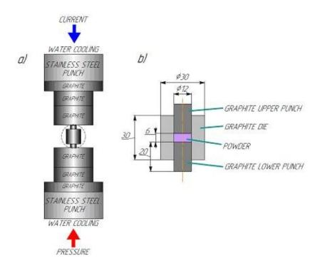
Schematic of the Spark Plasma Sintering apparatus: general scheme (a); sample placement in a mold (b). Credit: Lobachevsky University
