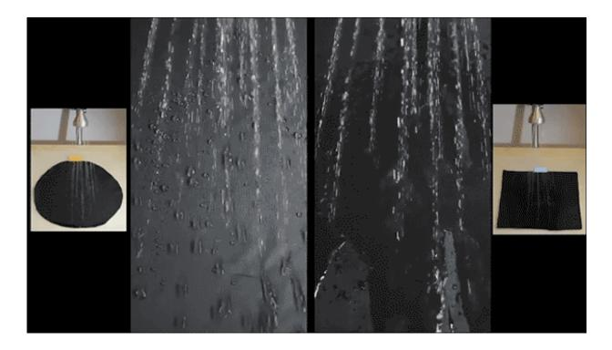
Testing of the coated surfaces shows that it gets a perfect score on a standard rain-repellancy test. The coatings are suited for substrates as diverse as fabrics, paper, and nanotextured silicon. Credit: Varanasi and Gleason research groups
