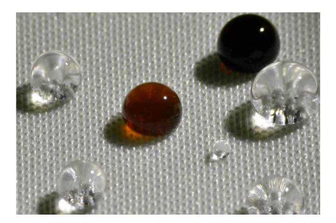
Repellency of different liquids on polyester fabric coated with H1F7Ma-co-DVB: soy sauce (black drop), coffee (brown drop), HCl acid (top left transparent drop), NaOH (bottom right transparent drop) and water (remaining transparent drops). Credit: Varanasi and Gleason research groups
