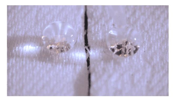
Comparison of droplets on a coated surface (left) and an untreated one (right). Credit: Varanasi and Gleason research groups
