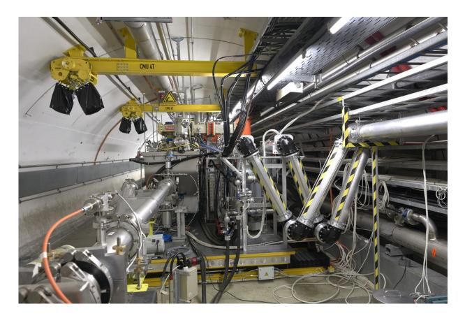
Crab cavity test in the SPS tunnel. Credit: CERN
