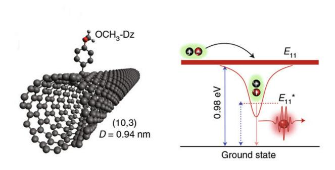
Depiction of a carbon nanotube defect site generated by functionalization of a nanotube with a simple organic molecule. Altering the electronic structure at the defect enables room-temperature single photon emission at telecom wavelengths. Credit: Los Alamos National Laboratory
