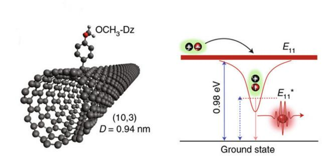
Depiction of a carbon nanotube defect site generated by functionalization of a nanotube with a simple organic molecule. Altering the electronic structure at the defect enables room-temperature single photon emission at telecom wavelengths. Credit: Los Alamos National Laboratory
