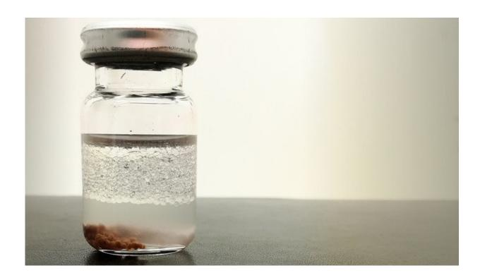
Biocatalysts (pictured at the bottom of the vial), supported by spherical lignin particles and embedded in natural polymer matrix, open new avenues to green synthesis reactions in the presence of water. Credit: Valeria Azovskaya
